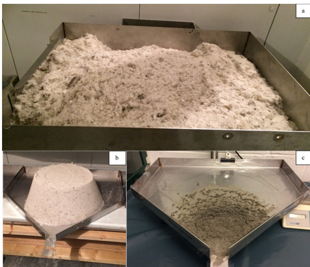
Figure 5. Image of a melting roadside snow sample in the laboratory showing presence of coarse sediments.
