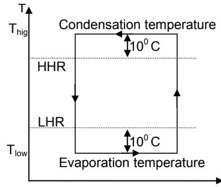
Fig. 6. Carnot Cycle of heat pump
