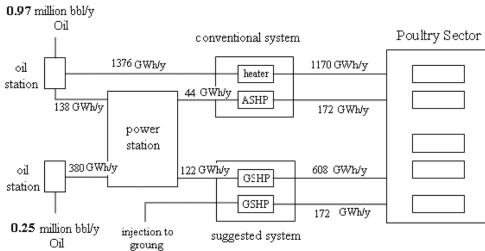
Fig. 15. Comparison between conventional and suggested system
