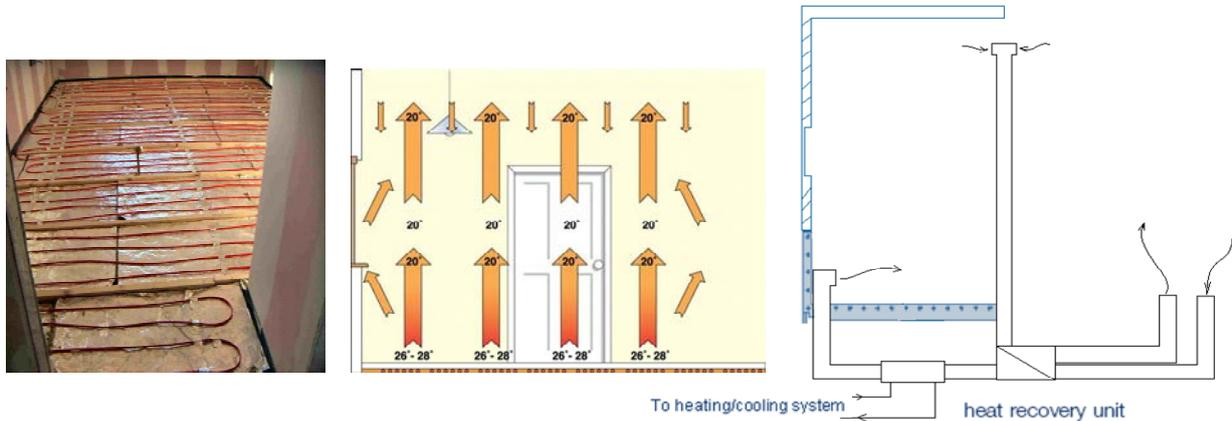
Fig. 13. Floor and wall heating/cooling distribution
