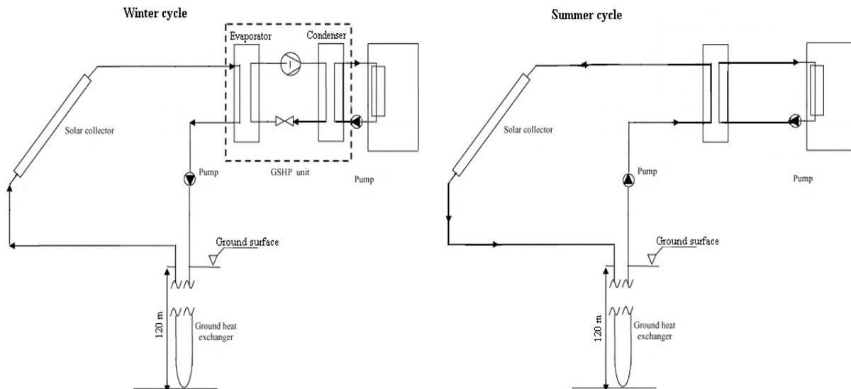
Fig. 14. Schematic of the solar coupled to ground source heat pump system.
