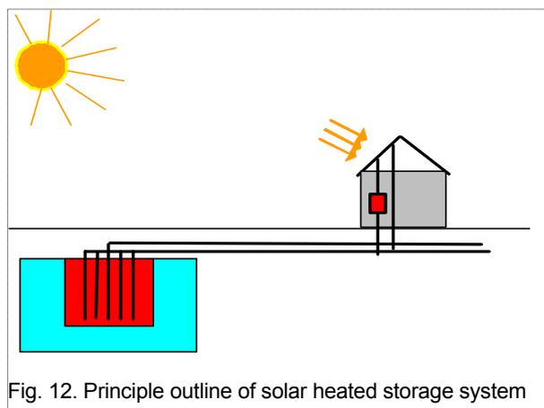
Fig. 12. Principle outline of solar heated storage system
