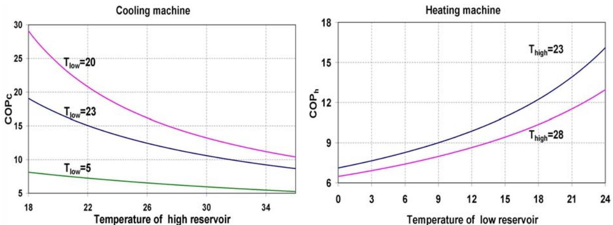
Fig. 7. COP as a function of low/high reservoir temperature.
