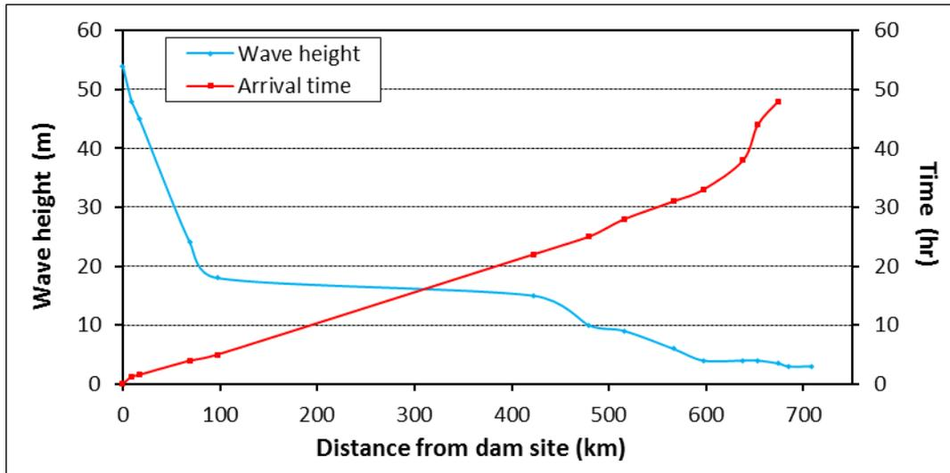
**Figure 2:** Water wave height due to Mosul Dam failure and time of arrival from the dam site downstream.
