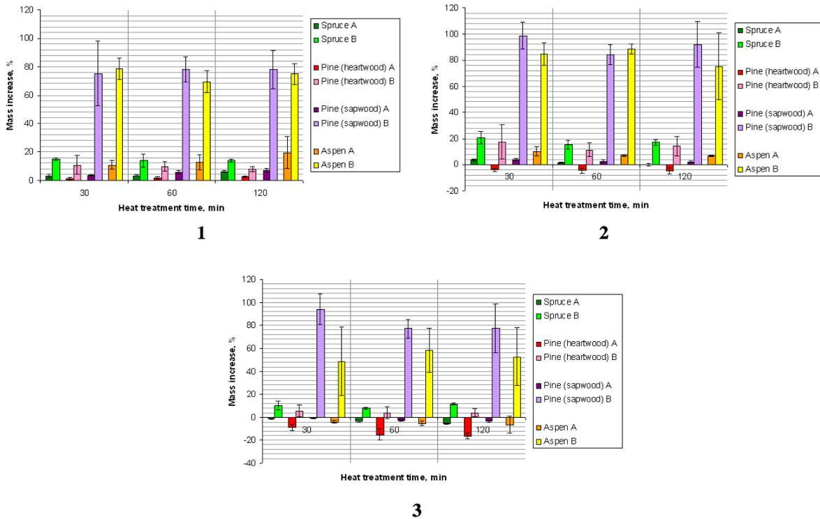
**Fig. 2: Mass increase during heat treatment and direct cooling in the oil bath (1 - Heat treatment at 180°C, 2 - 210°C, 3 - 240°C. Spruce A, Pine A, Aspen A – samples cooled in the air after heat treatment; Spruce B, Pine B, Aspen B – samples cooled in the oil bath after heat treatment).**
