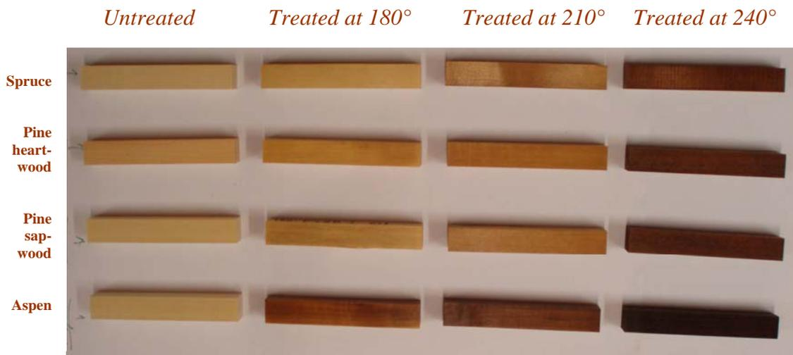
**Fig. 3: Samples before and after heat treatment**
