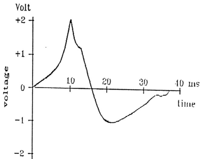
*Figure 6. Typical graph of the voltage curve obtained by frequent knockings (using the fist) on top of the test bone.*
