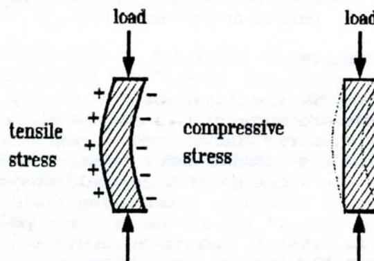
Figure 4. Bone subjected to a mechanical load generates an electric potential between the compressed and the stretched side of the bone (left). As a consequence of the electric potential bone is deformed on the compressed side resulting in an optimized stress load of the bone (right). After Herbst (1982).
