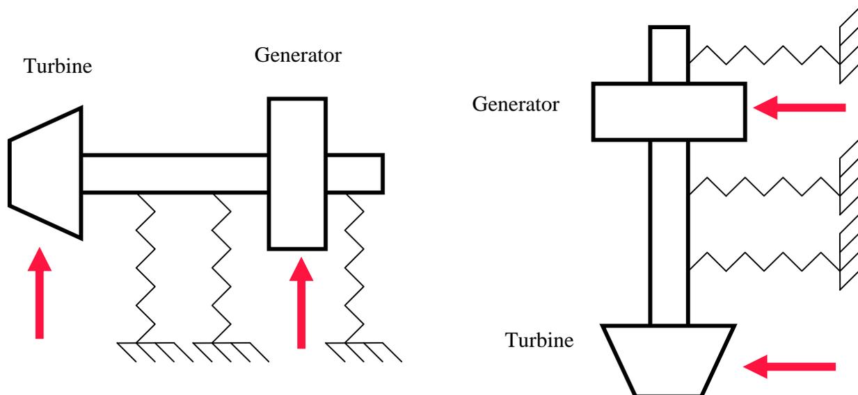
Figure 1, To the left an ordinary horizontal machine and to the right a typical hydro power rotor. Red arrows marks forces from fluid and electro magnetic fields.
