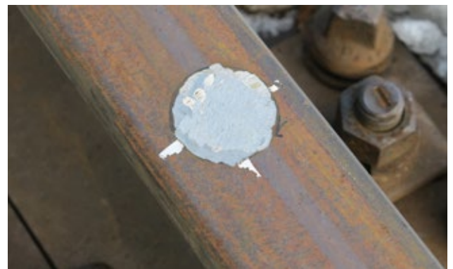
Figure 6. Artificial introduced realistic squats as input to AI.
