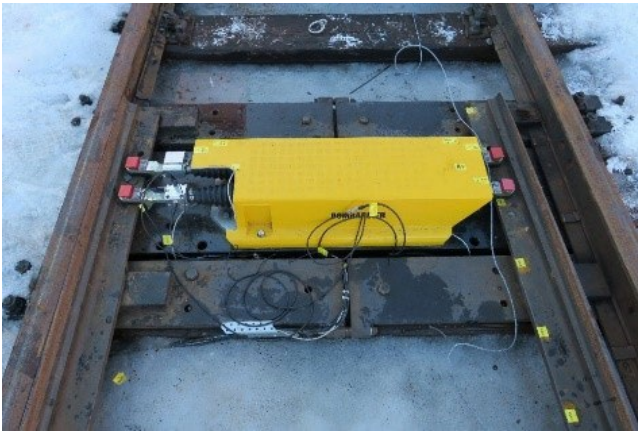
Figure 2. Point machine with assembled vibration sensors used in the study.
