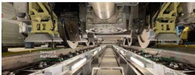
Figure 1. Differential eddy current measurement system mounted on both sides of a freight train.
