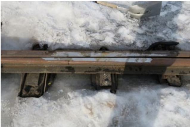
Figure 4. Artificial introduced realistic wear on support rail as input to AI.
