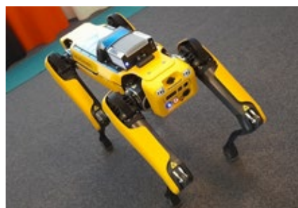
Charlie the robotic dog that carries sensors for monitoring and inspection.
