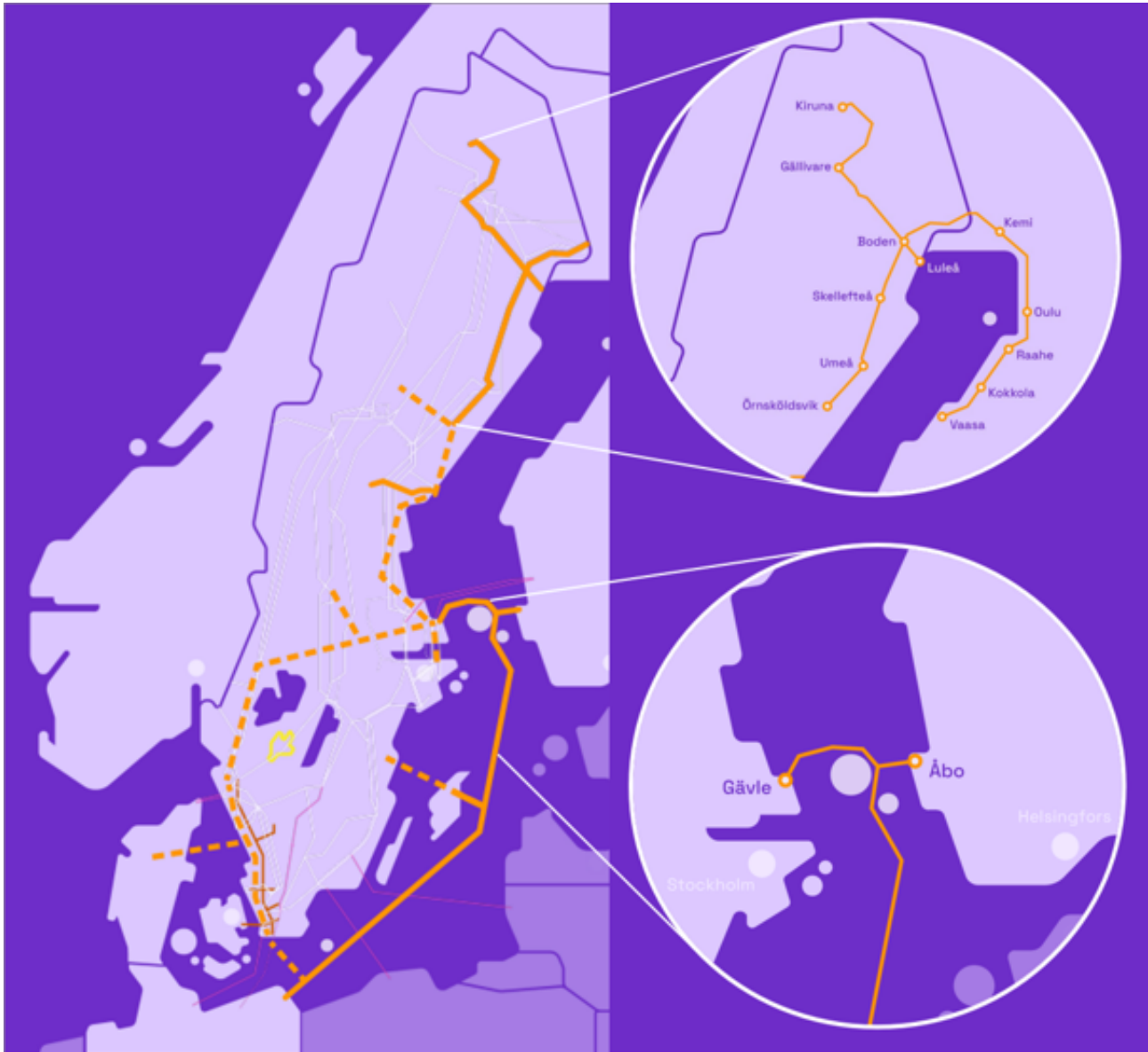
Figure 5: Hydrogen gas grid. Solid orange = Planned hydrogen networks, Dotted orange = Future hydrogen network, Dark orange = Current gas grid, Yellow = Electricity grid (Source: Nordion presentation)
